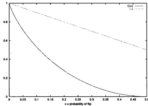
Figure 7: Capacity and 1-BER, plotted against BER
